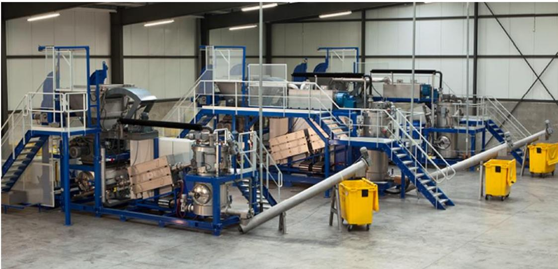
Figure 18 Installation machines Ecosteryl (Source : <https://cosmolys.com/solution-globale/> )
